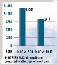
This chart compares the 5-year savings you can expect from an AC13 air conditioner vs. units with lower efficiency ratings, based on a 36,000 Btuh/3-ton unit (EPA Region 9). Your actual savings will vary depending on the weather, local fuel rates, indoor coil and your lifestyle.
